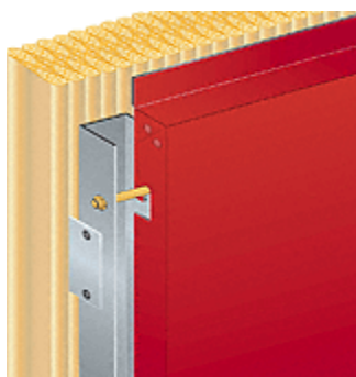
«Construction example ۵» Tray panels Suspended on stainless steel bolts Vertical panel layout
