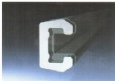
Special Profiles as Tensioning Shoes used in Precision Clamping Tools In the past, these were based on forged blanks. The subsequent compulsory and essential all-around machining of that blank was completely eliminated by the change to a special profile.
