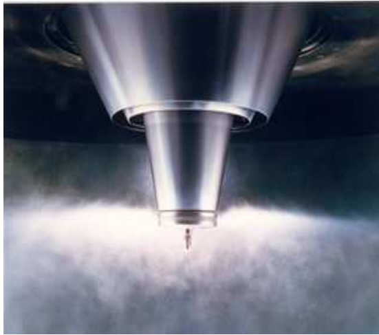
Rotary atomizer in a spray dryer
