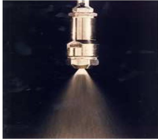
Nozzle atomizer in a spray dryer
